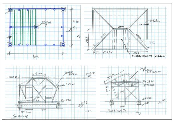
**Figure 1.1 – Sketches of Shelter Geometry**
