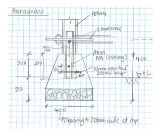
**Figure 1.3 – Foundation Detail**
